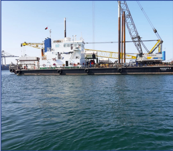
Ghumays II -self-propelled crane barge
